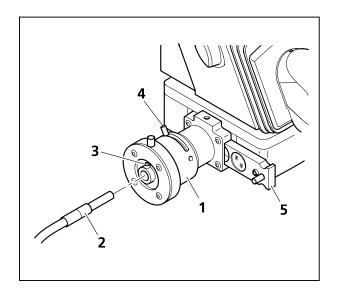
Fig. 23 Connecting the optical fiber of the X-Cite illuminator to the PentaFluar S/X-Cite
