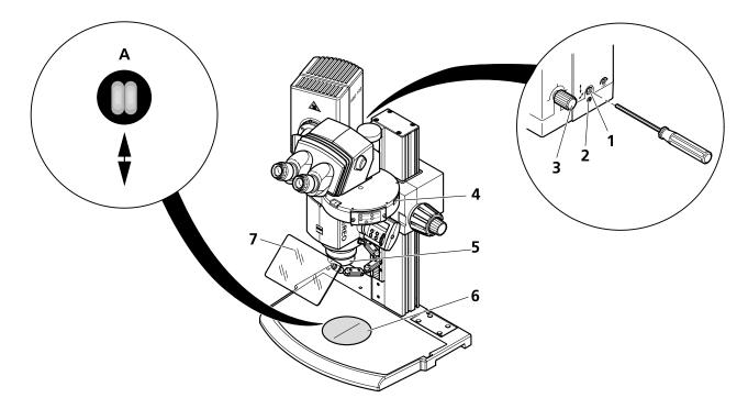
Fig. 35 Adjusting the HBO 100 illuminator
