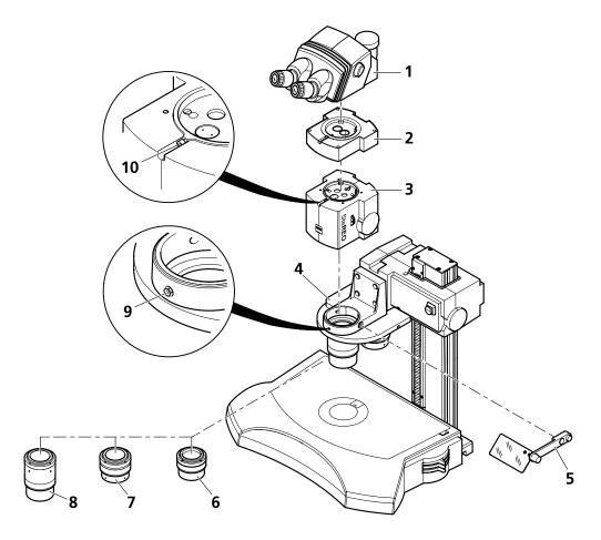
Fig. 15 Installing the microscope
