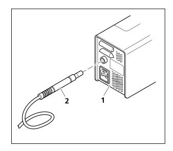
Fig. 24 Connecting the optical fiber to the X-Cite illuminator
