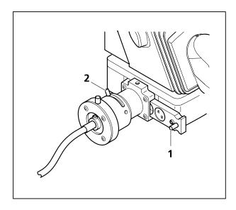
Fig. 34 Adjusting the vertical illuminator
