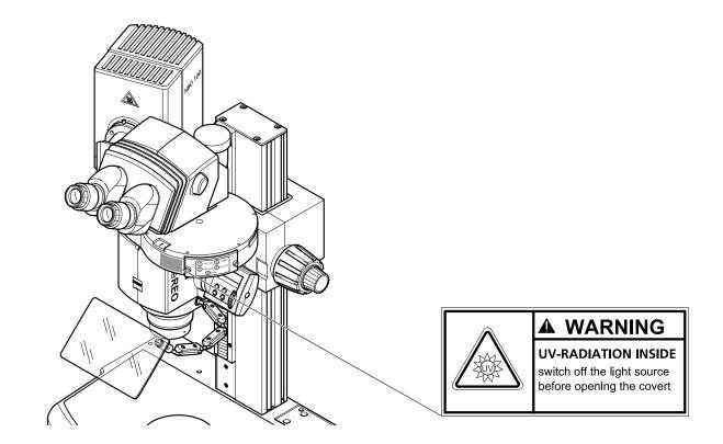
Fig. 2 Warning label on PentaFluar S vertical illuminator
