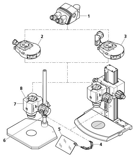
Fig. 21 Installation of PentaFluar S/X-Cite or S/HBO
