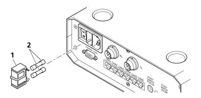
Fig. 41 Replacing the fuse on the EMS-2
