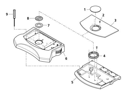
Fig. 13 Installing the transmitted-light equipment S
