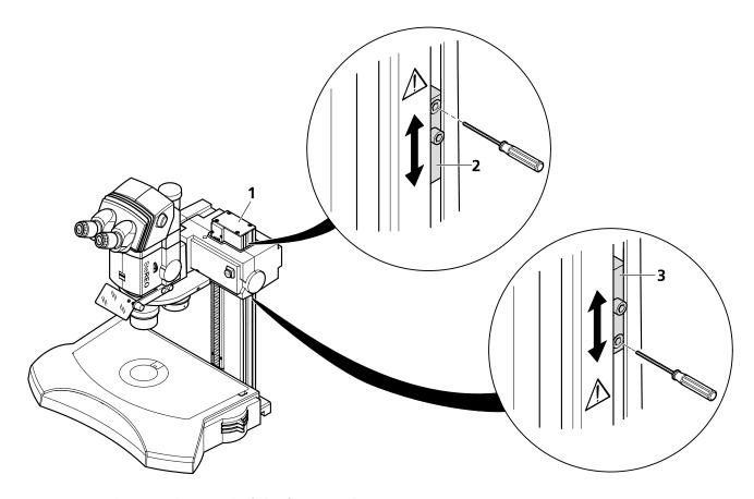
Fig. 28 Adjusting the travel of the focusing drive
