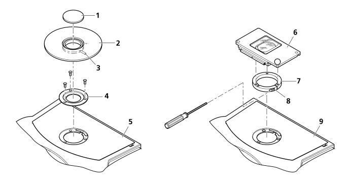
Fig. 14 Installing the stage
