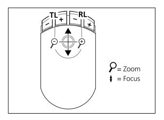
Fig. 39 Functional elements on SYCOP
