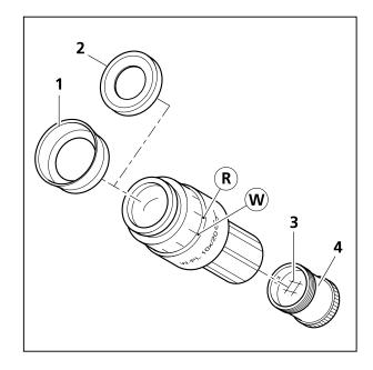
Fig. 16 Inserting the eyepiece reticle
