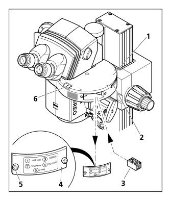
Fig. 22 Inserting filter blocks
