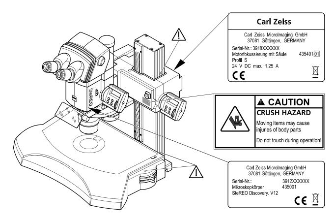
Fig. 1 Warning and information labels on the instrument
