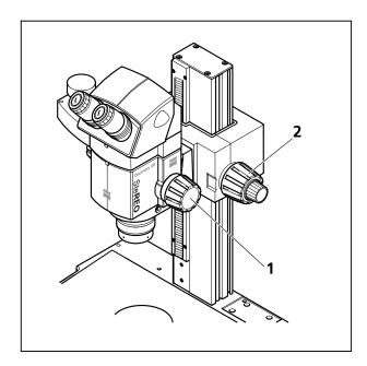
Fig. 31 Adjusting the stereomicroscope (manual zoom and focusing, e.g. SteREO Discovery.V8)
