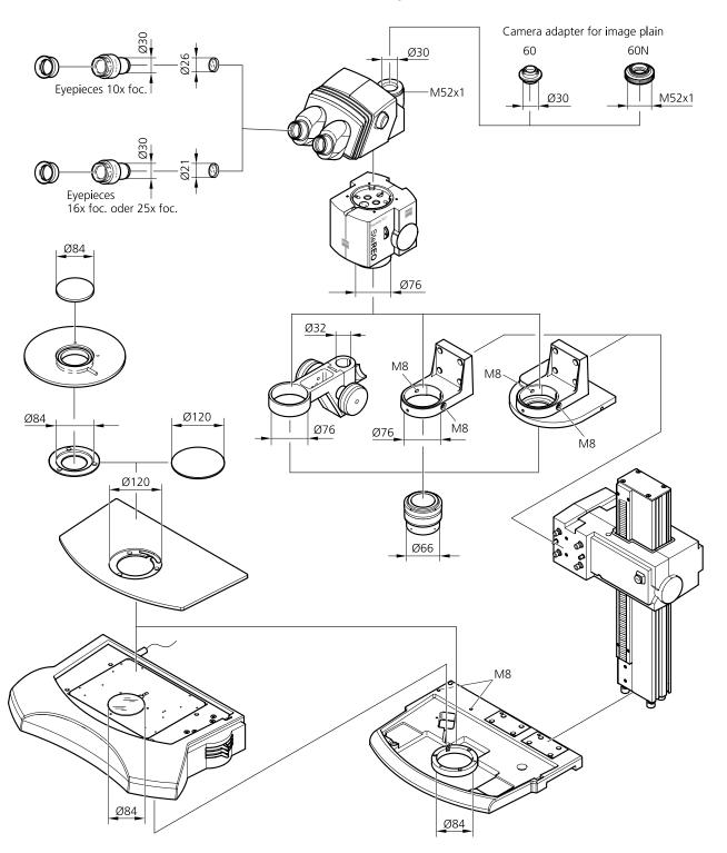
Fig. 11 Mechanical interfaces on SteREO Discovery
