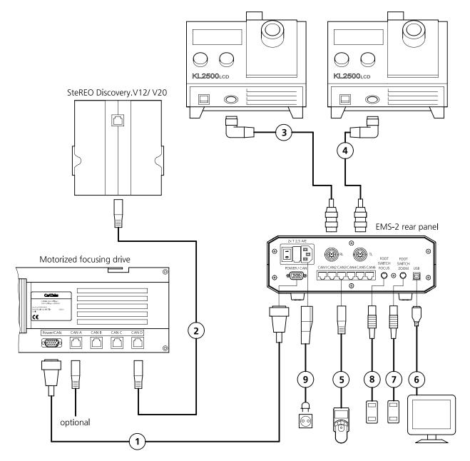
Fig. 27 Connecting the SteREO microscope
