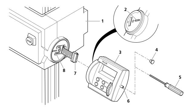
Fig. 26 Installing the HIP control unit
