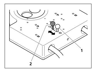
Fig. 32 Switching lever for optimising the illumination of the specimen field (mounted at the bottom side)
