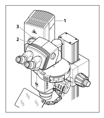
Fig. 25 Connecting the HBO 100 illuminator to the PentaFluar S/HBO 100
