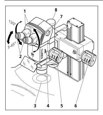
Fig. 30 Adjusting the stereomicroscope (motorized zoom and focusing)
