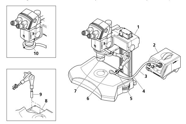
Fig. 18 Installing the incident-light illuminator
