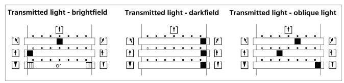
Fig. 29 Setting illumination control on transmitted-light equipment
