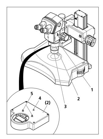
Fig. 20 Coaxial epi-illumination (upper side)
